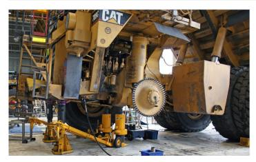
The EDMO Lift'n'Lock is an Air Hydraulic Jack and Locking Support Stand combined in one unit. It complies with both the Australian Standard for Jacks and the Australian Standard for Vehicle Stands.
