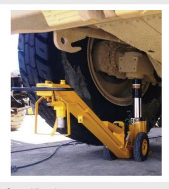
The EDMO DMA200 is a single stage hydraulic jack, powered by an air pump. Like all EDMO Jacks, the DMA200 far exceeds the minimum safety standards required by AS/NZ2693. The DMA200 is fitted with a self drive 'motivator' unit (EDMOTIVATOR) to assist in moving the unit into position.
