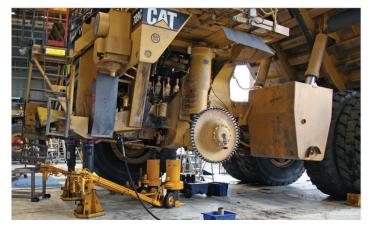
The Transporter has a spigot which fits into the socket of the stand. By pushing down on the end at the handle, the stand will be picked up enabling movement and positioning from a greater distance. To release the stand, the handle of the Transporter is lifted and pulled away from the stand to disengage from the spigot.
