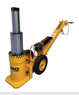
This is a 2 stage hydraulic jack powered by an air pump. It is operated from the end of handle, away from the jack operations. The jack is power up and power down. Safety is a feature of the UPDT100/50 having a pilot operated lowering control valve which requires the Jack to be pumped down thus providing protection against a free fall and gives complete control over the lowering process.
