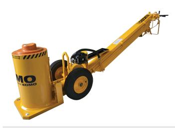
This is a 2 stage hydraulic jack powered by an air pump. It is operated from the handle, well clear of the load. The jack is power up and power down. The EDMO PDT200/100 Jack comes fitted with the self-drive EDMOtivator unit, to assist in moving the unit into position.
