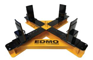
The EDMO Adjustable Rim Stand is fabricated with the quality and high standard of workmanship associated with the EDMO brand. It is designed for supporting Earthmover wheel rims during maintenance and repairs. Adjustments to suit the rim size are made by sliding the stops and bolting them into position. A centred lifting lug provides a lift point for easy transport around the workplace.
