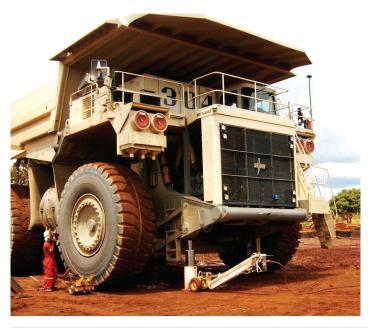
The EDMO TPDT150/75 is a 2-stage hydraulic jack powered by an air pump. Operating controls are on the handle, well away from the jack body. The jack is power up and power down.
