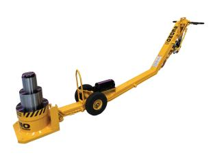
The EDMO UPDT100/50 is a low line jack, one of the smallest in the range. Its low-line design is for those situations where ground clearance is small. This feature is particularly useful for underground machinery and any other equipment with low clearance such as water trucks. The Jack only requires air supply of around 100 psi for its operation. The unit is completely self-contained and is very easily maneuvered into position or around the workshop.
