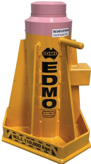
Specially designed for the D10 & D11 dozers, the EDMO DS110-635 is a rigid stand with a smaller base area to allow for better positioning under the pivot pin and clearance for the removal of the tracks.
